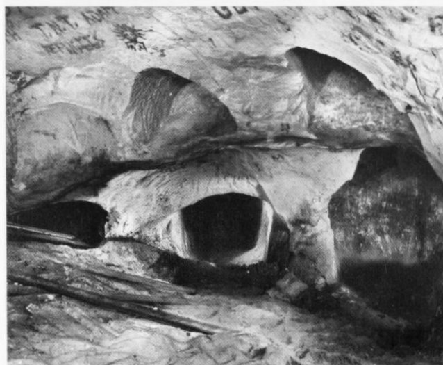
London Road mine: silver-sand extraction on two levels can be seen here, separated by a hard band of iron-cemented sandstone. Where this material, called 'carstone' or 'brown flint', has been taken out of the mine it has been used in and around the Reigate Castle grounds for hard-wearing surfaces for footpaths and steps. Qualities of sand from pure white to heavily iron-stained can be seen. The whitest material would have made clear glass. Depending on the iron content, lesser grades would have been suitable for making brown or green beer bottles, or as builders' sand.
